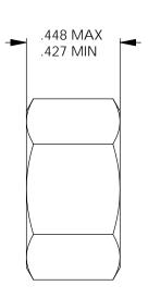
1/2"-13 UNC HEX NUT - TAPPED .018 OVERSIZED MUST CONFORM TO ALUMA-FORM SPECIFICATION #90005
